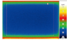
Dark signal non-uniformity (of the system without correction) at 5 s integration time and 25 °C
